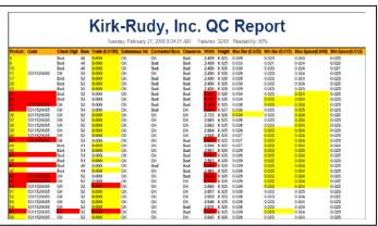
Keep tabs of each job and the number of failures using the QC System's report generator. The report lists each marginal and failed barcode along with its parameters. Warning items are highlighted in yellow while failures are highlighted in red.
