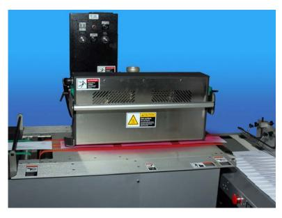
Specially designed bulbs reduce glare and direct most infrared energy towards the ink pattern. This means lower power settings can be used, reducing energy consumption and extending bulb life.
