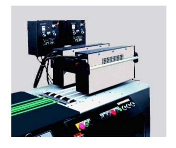
Add an additional KR 881 for drying two separate lnk patterns or one wide pattern.
