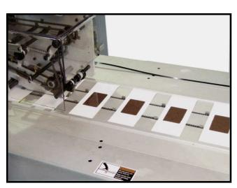
Pusher lugs on the transport and the attaching head ensure product is straight during the attaching process.
