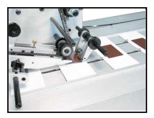
Cards are individually fed, squared and registered on the card attaching head. Pusher lugs keep the card straight throughout the attaching process. Press down rollers secure the card in place.
