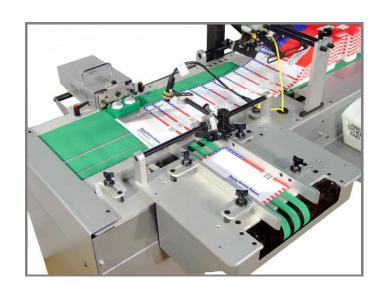
The KR 345's high-speed infeed table and clutched conveyor belts ensure a neat, consistent shingle.
