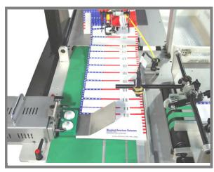
The KR 345 shingles mail in the conventional manner. Conveyor belts stop when the flow of product entering the machine stops keeping the shingle consistent. A two-position backstop offsets the shingle indicating zip and bundle breaks.
