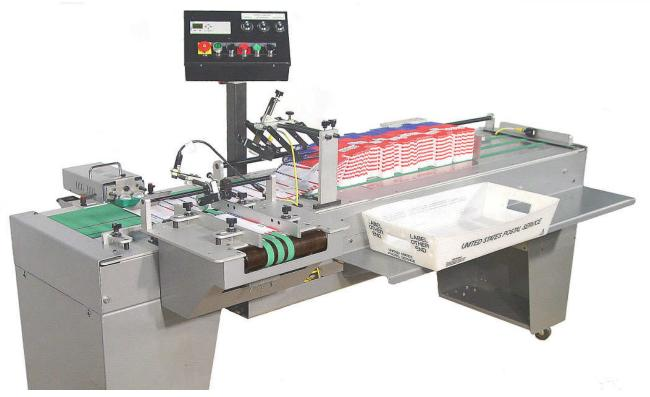
An all-new concept in mail handling, the KR 345 takes the hassle out of sorting and traying mail. Part shingle conveyor, part edge stacker, the KR 345 combines the advantages of each system into a simple, laborsaving unit.
